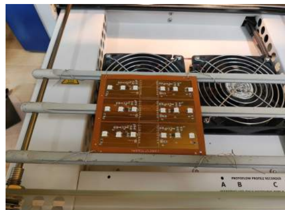
Figure 6: Flex PCB secured with wire
