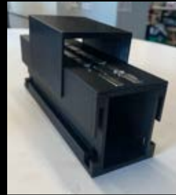
Track - 2.5cm rectangle magnets - no spacing
