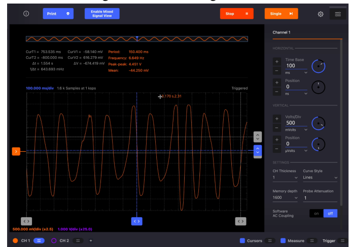
Fig. 9. Induced EMF in the Faraday's law experiment.
