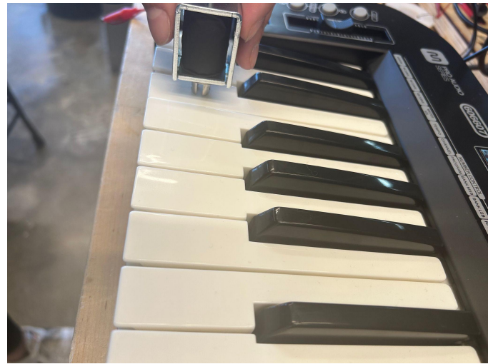
Fig. 6 (c) The location of the solenoid in relation to the keyboard
