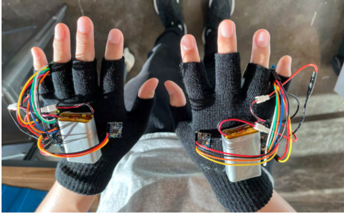
Fig. 6. Two gloves are identical. Right hand (right) will include a color coded middle finger for position tracking color detection when the product is in use. The color of the middle finger will be determined based on the color of the user's shirt.
