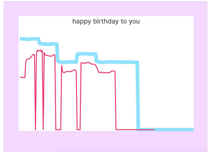
Fig. 2. A screenshot from the KaraoKey app displaying the main feedback mechanism. The user's pitch (in red) is plotted against the target pitch (in blue).
