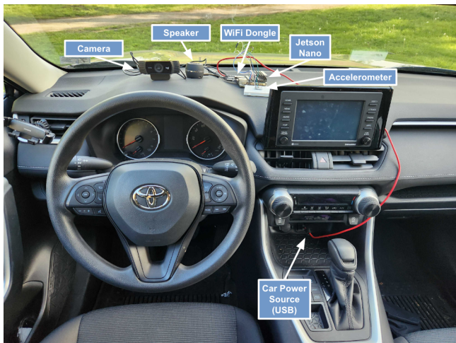
Fig. 1. This is the setup of the DriveWise device in an actual car.
