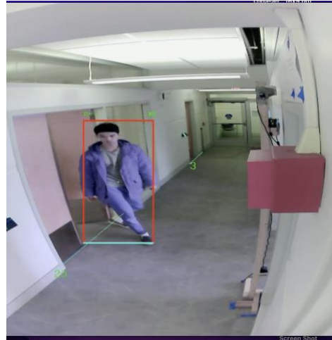
Fig. 4. People Counter's CV output bounding box of a person
