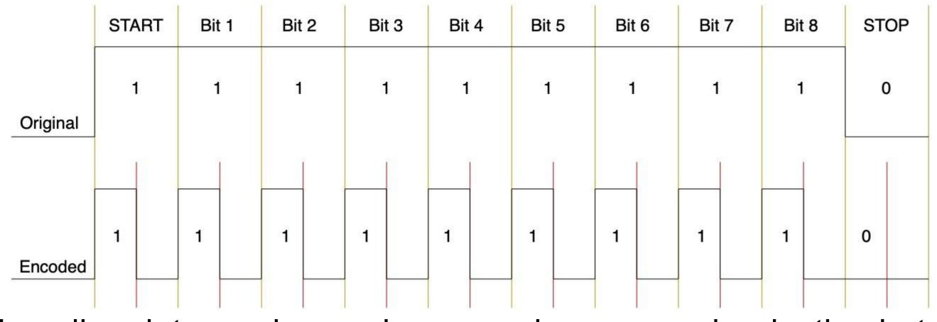
Encoding data as shown above requires a speed reduction but allows for ambient light filtering for operation in varying lighting.
