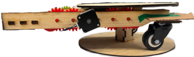
Fig. 6.3. Side view of the lift arms midway through the docking sequence
