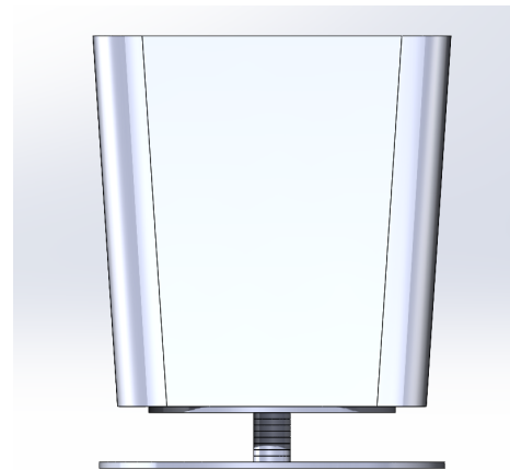
Fig. 5. Side view of the modified trash bin showing the bin, upper disk, central column, and lower disk (from top to bottom).
