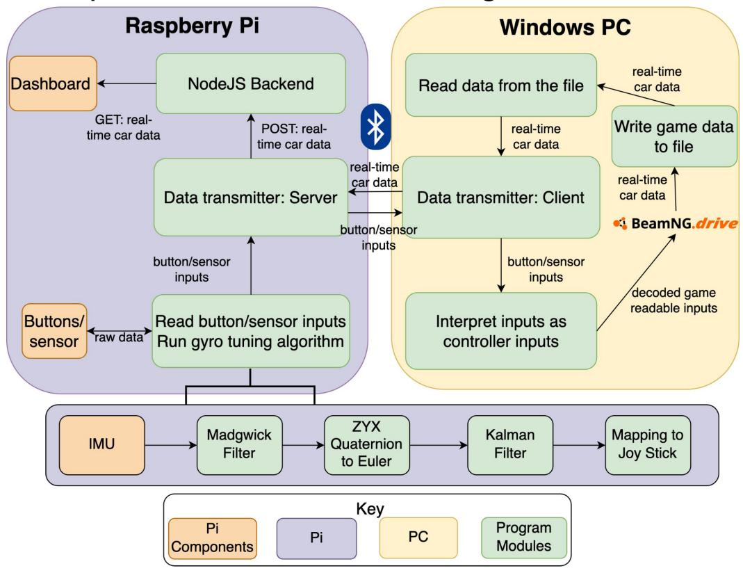
Controller data is transmitted through Bluetooth to PC to control the game. Game data is sent back from PC to Pi to display car information on dashboard.
