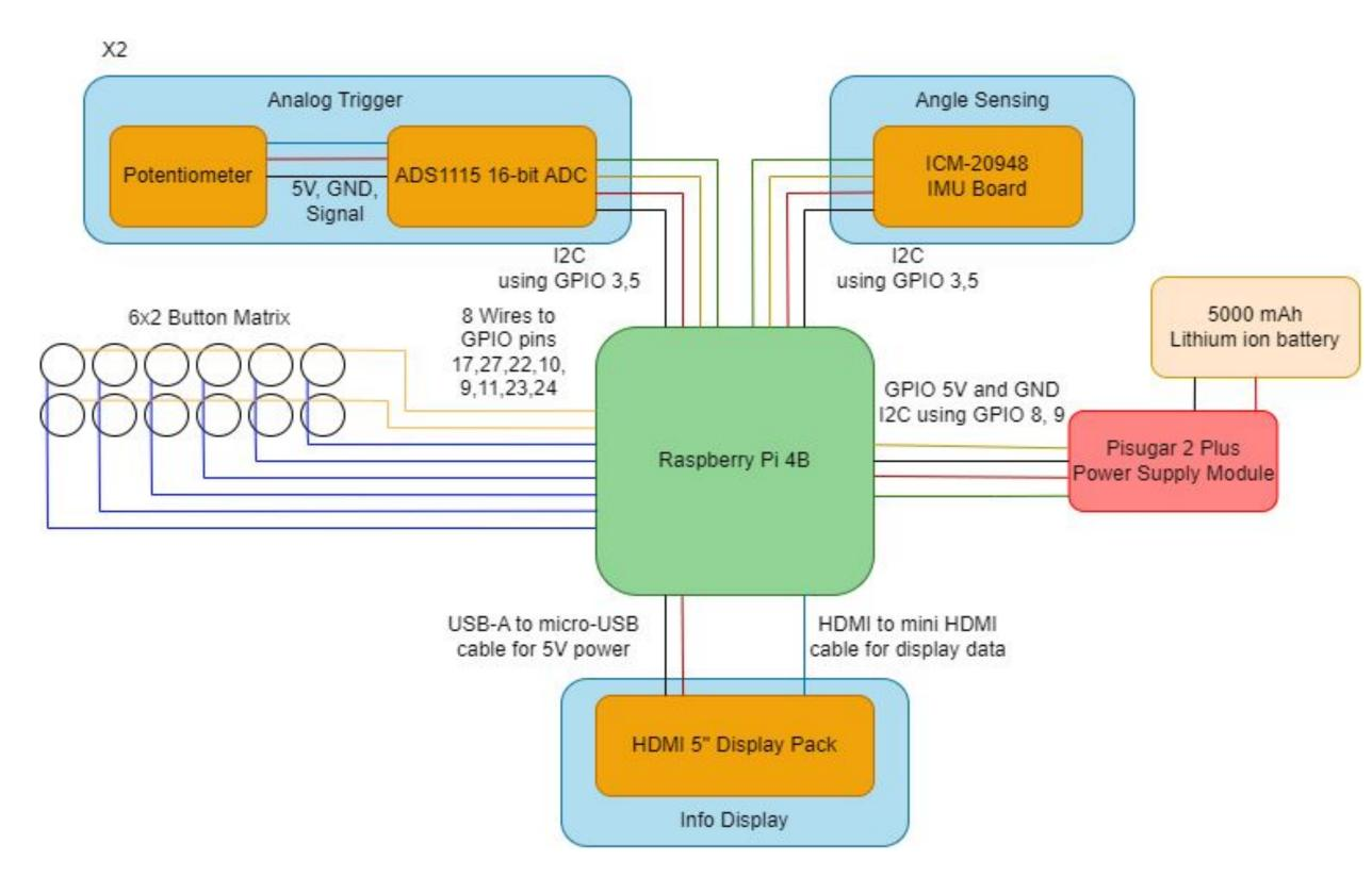
The hardware system (picture above) consists of all off the shelf components, with custom wiring.
