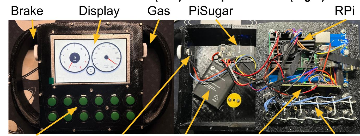
Buttons Encoder Battery IMU & ADC Buttons
