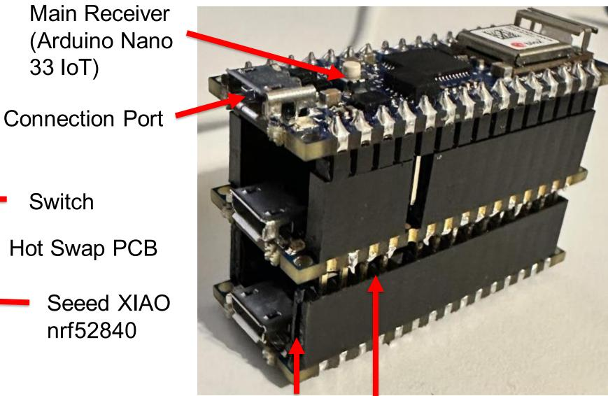
Auxillary Receivers 1 & 2 (Arduino Nano 33 BLE)
