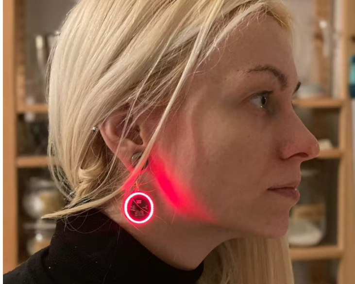
HALO-90 open source earrings: uses 90 single-color red 0402 diodes, STM8L151G4 microcontroller, CR2032 coin battery, microphone & button
