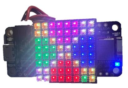
The firmware uses Adafruit's BLE and DotStarMatrix libraries to achieve Bluetooth communication and easy control over the LED matrix. We have two versions of firmware that allow user to use either our own app or the Adafruit's BLE app (downloadable from App Store) to interface with the LED matrix wirelessly.
