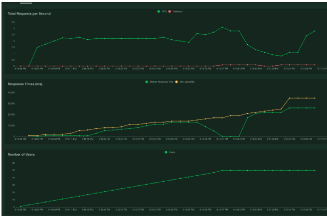
Fig. 5. Using the Python Locust library, these are the Load-testing results of our WebApp that is hosted on an EC2 instance on the AWS free tier. Because of such, we can see that HTTP failures and server response times increase as user requests approach our defined capacity limit of 50 users.
