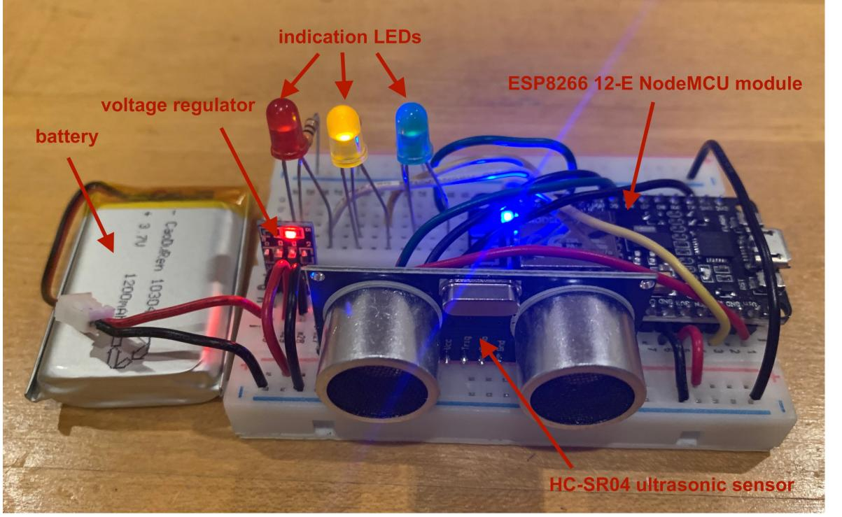
Kerby's spot modules are placed on the curbside, distanced at 8 feet apart. When 3 sensors are detected as free, then an open spot is determined and displayed on the web page.
