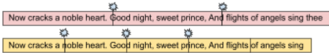
Fig. 2. This figure illustrates the problem of fixed-sized chunking. Simply changing the chunk size does not remove the probability of cutting off a spoken word.
