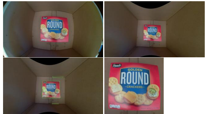
Fig. 11. Showcase of the CV processing. Initial raw image taken by RPI, top left. Undistorted image, top right. Image with annotated regions of change, lower left. Localized image, lower right.
