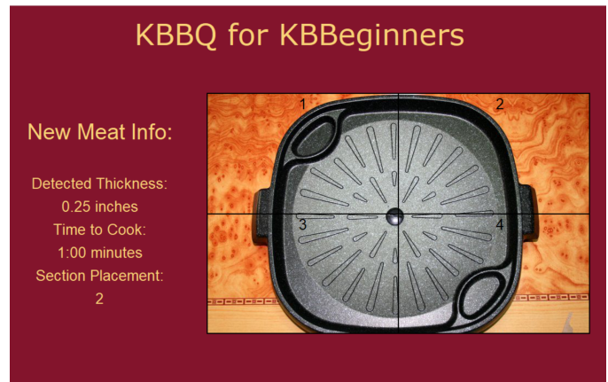
Figure 9: Layout of UI design. The mentioned camera feed is on the right, while information on the newest meat to be put on the grill is on the left.
