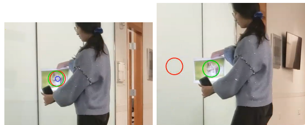
Figure 5: KLT test with the red circle indicating the initial position of the target (Tamal the squirrel), and the green circle indicating the tracker's prediction of the target's new location.
