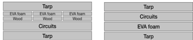
Figure 8: Different arrangement of layers of tarp and EVA foam for game mat
