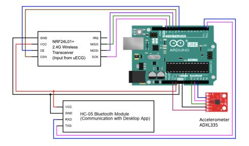
Fig. 3. Wiring diagram for the components inside the belt clipped device. Inside the belt-clipped device there will be a wireless receiver for the uECG device, an accelerometer, and a bluetooth module to communicate with the desktop app.
