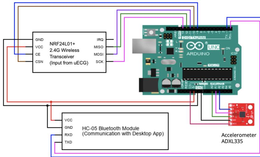
Fig. 3. Wiring diagram for the components inside the belt clipped device. Inside the belt-clipped device there will be a wireless receiver for the uECG device, an accelerometer, and a bluetooth module to communicate with the desktop app.
