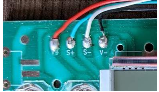
Figure 6: Load Cell Connection to NEXT-SHINE kitchen scale
