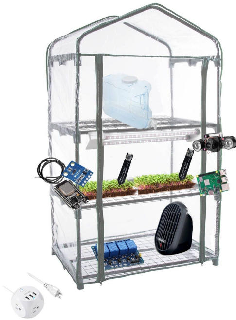
Fig. 1. Overall system design of the greenhouse (Images are from Amazon product description pages)
