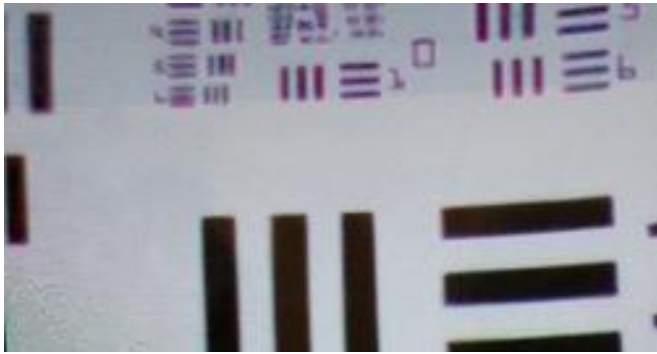
Fig.11. MTF test with a close-up crop of the test card showing the bottom-left 6 being the smallest part of the lines that can be discerned between.
