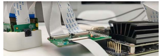
Fig 2. Camera Subsystem & Jetson Nano Interface 4
