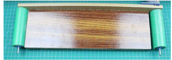
Fig 4. Partially Completed Conveyor Belt System 6
