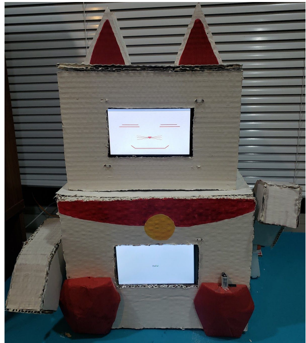
Fig. 10. Completed Custom-made Robot. The robot is constructed out of cardboard, and other household items due to lack of access to 3D-printing and laser cutting during remote instruction.
