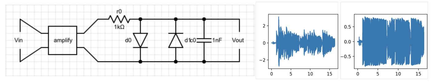
**Circuit Simulator:** The circuit simulator obtains a stream of voltages from the audio processor. For each voltage, KCL is performed at each node to produce a system of equations, which solved using Gauss-Jordan Elimination.
