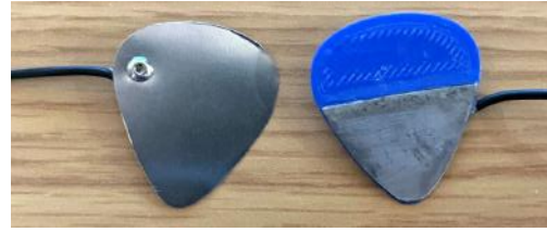
Fig. 13. Guitar picks with metal electrodes. The left pick has an electrode on both sides, while the right pick only has an electrode on one side. They can be easily interchanged to match the user's preference.
