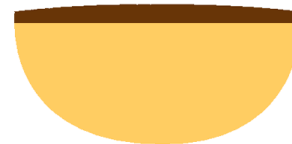
Fig. 6. Cross section of a guitar fretboard. The fretboard surface is curved, making PCB mounting difficult [7].
