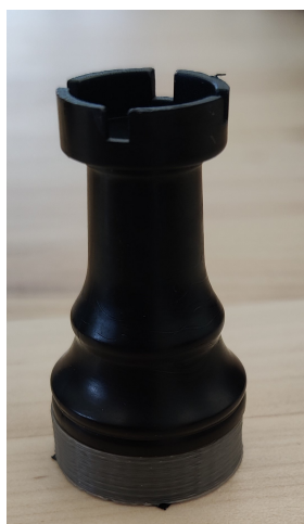
Figure 2: An example of a modified chess piece with a 3D printed holder for the magnet underneath
