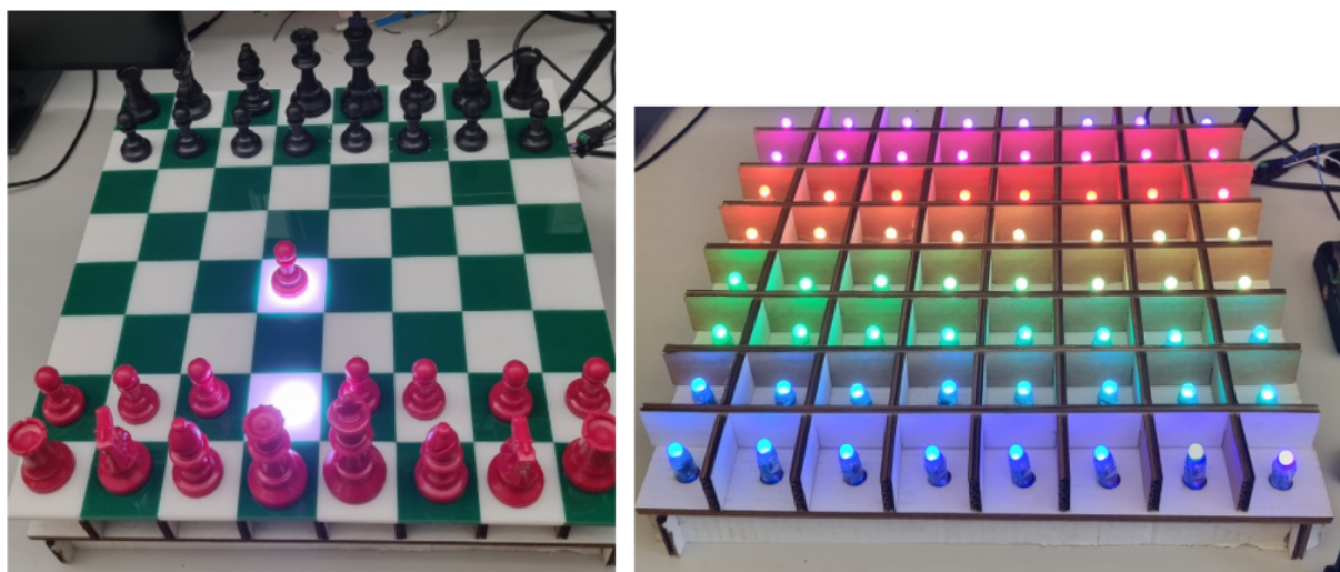
Figure 4: Image of the final board (left) and LED matrix (right)
