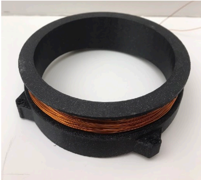
19. Custom made RFID antenna coil wrapped around custom designed and 3D printed frame
