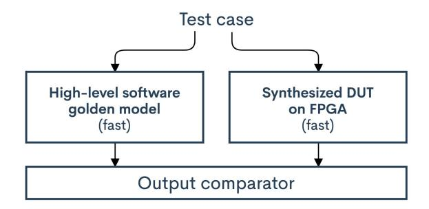
The DUT will be a single-cycle RISC processor with a limited instruction set.
