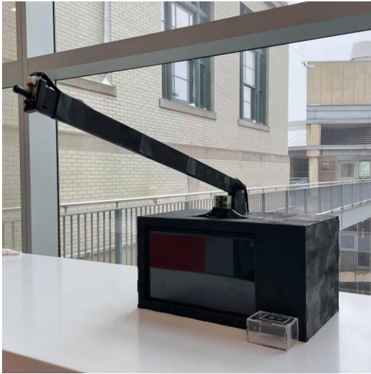
Fig. 16. Final laser cut and painted product.
