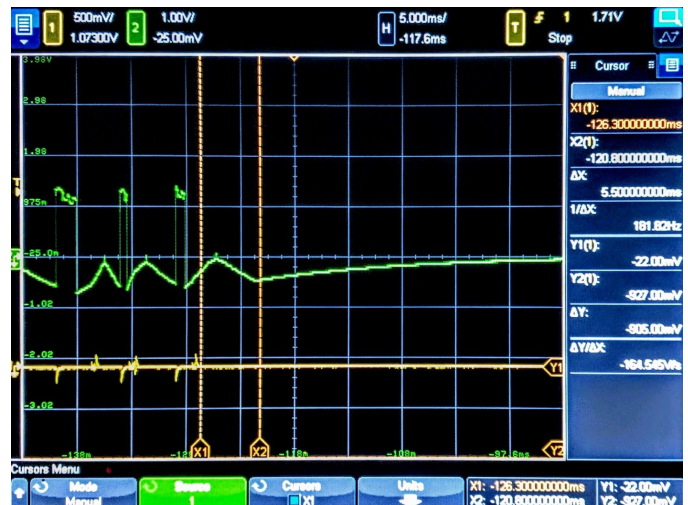
Fig. 5. Response time between DAC stall and laser shutdown.
