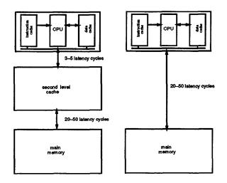
Figure 1: Basic implementations of microprocessor based systems
