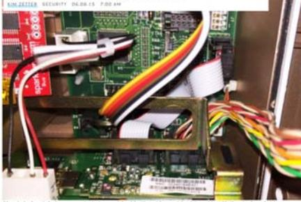
Hospitals' drug infusion pumps include a serial cable (the wide grayish-white cable with the single red stripe on one edge) that connects the communications module to the main pump board. Because the libraries don't require authentication, Risos found that anyone on the hospital's network—including patients in the hospital or a hacker accessing the pumps over the Internet—can load a new drug library that alters the limits for a drug.
