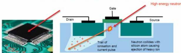
Radiation strike causing transistor disruption [Gorini 2012].
