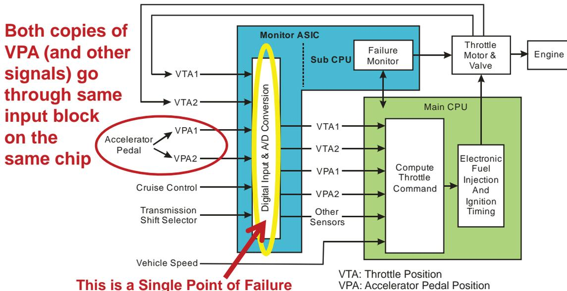
This is a Single Point of Failure
