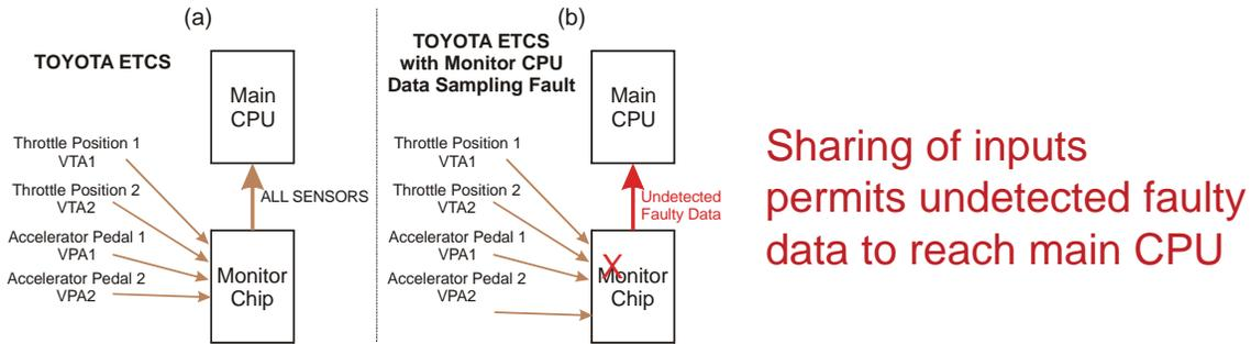
Alternate design uses separate A/D inputs to cross-check data
