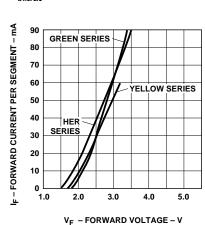
Figure 11. Forward Current vs. Forward Voltage.
