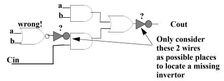
To keep the algebra simpler, only consider the 2 wires shown above as possible locations for the missing invertor. Note--you know what the right answer is by looking at this problem--but the point is to show how, by using purely Boolean manipulations, you can identify the right invertor to add. Show any extra logic you need to add to make the network you need to apply quantification to. Show all the steps of the analysis.
