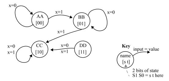
The machine above has four states AA BB CC DD, represented by 2 bits of state (2 flip flops) whose values appear in brackets (e.g., [10] represents state CC) in each state bubble. This machine has just 1 input x. We are ignoring any outputs for this machine.
